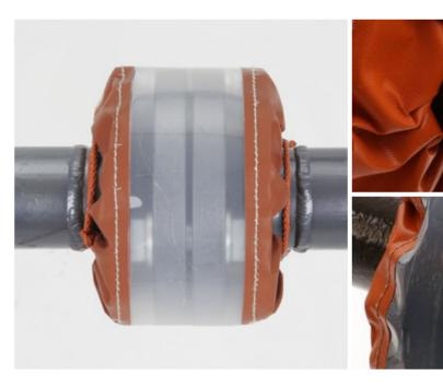
Flangeguards PTFE-CLEAR shield is manufactured from Teflon coated fibreglass PTFE, with wide central band of clear Teflon (ECTFE). This material is resistant to hydrocarbons and chemical liquids.
