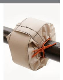
The multi-layered mesh held tight against the flange, forms the basis of our Pressure Diffusion Technology (PDT). The result is a selfdraining, incredibly effective way of preventing spray-outs (side or lateral) and mist formation.
